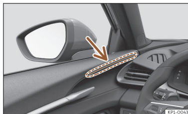
Fig. 167 Door: warning lamp
