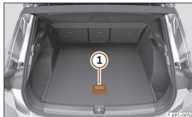
Fig. 186 Variable luggage compartment floor: high position.
