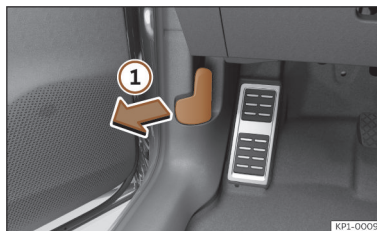
Fig. 221 Release lever in the driver's footwell area.
