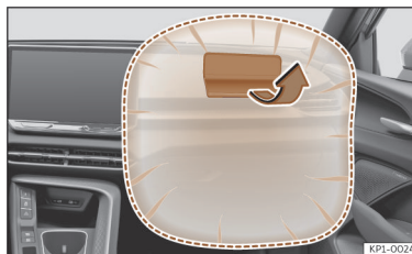
Fig. 29 Front passenger airbag located in dash panel.
