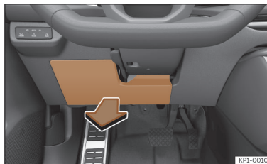
Fig. 217 On the dashboard on the driver side: lid of the fuse box.
