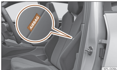
Fig. 34 Side airbag in driver's seat.
