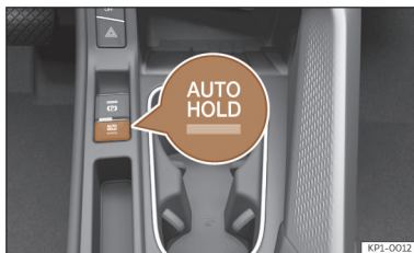
Fig. 149 In the lower part of the centre console: Auto Hold function button.
