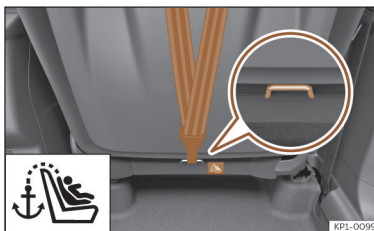
Fig. 44 Rear of front passenger seat backrest: Top Tether belt anchor (not available in all markets/versions).
