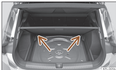
Fig. 188 Variable luggage compartment floor: tilted position.
