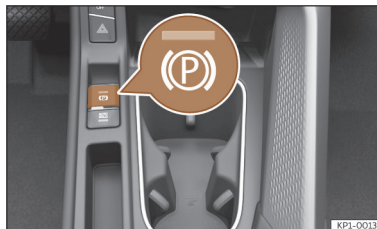
Fig. 148 Centre console, lower part: electronic parking brake button.
