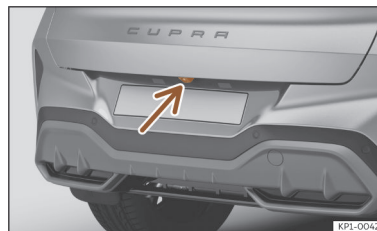
Fig. 129 On the rear lid handle: location of the rear assist camera.
