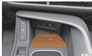
Fig. 181 On the centre console: pad for the mobile phone connection.
