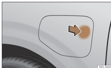
Fig. 57 Opening the charging socket cover.
