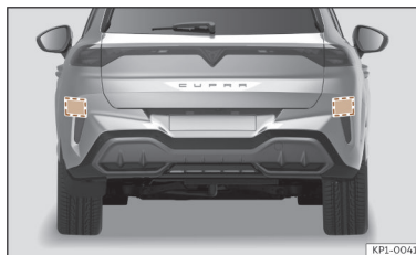
Fig. 127 Rear view of the vehicle: radar sensor areas.
