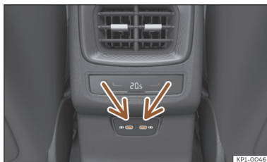
Fig. 175 Rear centre console: USB connectors with power socket function.
