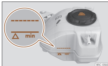
Fig. 224 In the front compartment: coolant expansion tank.
