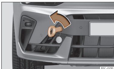
Fig. 216 Right side of the front bumper: towline anchorage screwed in.
