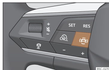
Fig. 130 Left side of the multifunction steering wheel: button for driver assistance systems (depending on the version).
