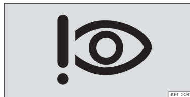
Fig. 8 On the instrument cluster display: Driver attention monitor symbol.
