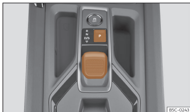
Fig. 126 On the centre console: selector lever.
