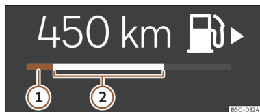
Fig. 3 Fuel gauge located in different positions depending on the view.
