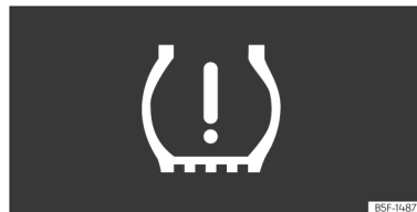
Fig. 247 Instrument cluster: warning of loss of tyre pressure.
