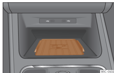
Fig. 185 On the centre console: pad for the mobile phone connection.
