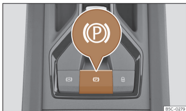
Fig. 156 Centre console, lower part: electronic parking brake button.
