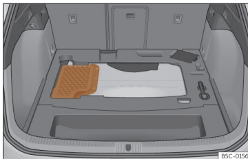
Fig. 234 Hybrid vehicles (PHEV): location of the battery in the luggage compartment
