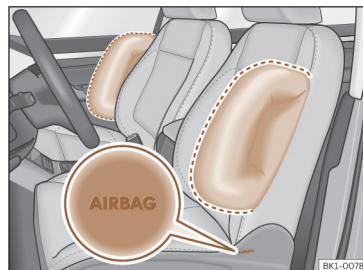
Fig. 32 Driver's seat and passenger seat side airbags.
