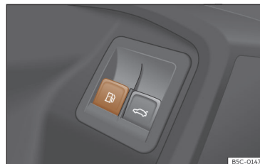
Fig. 206 Driver's door: tank flap release.
