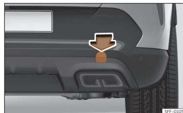
Fig. 217 Rear bumper on right: remove the lid.
