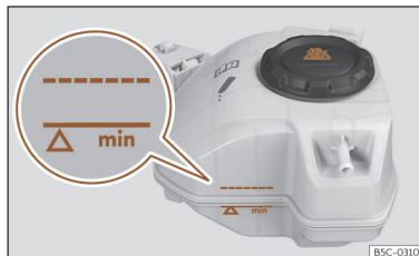
Fig. 225 In the front compartment: coolant expansion tank.
