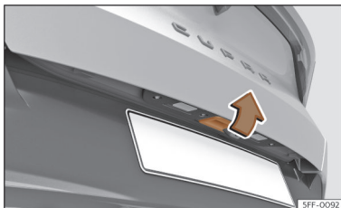
Fig. 83 Rear lid: opening from the outside.
