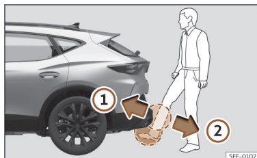
Fig. 86 Rear lid with sensor-controlled opening (Easy Open).
