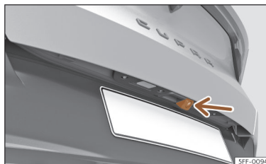
Fig. 136 On the rear lid handle: location of the rear assist camera.
