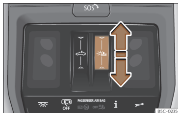
Fig. 92 On the headliner: operate the sun blind.
