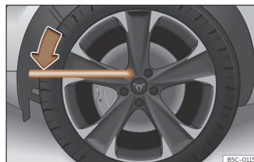
Fig. 244 Tyre change: loosen the wheel nuts.
