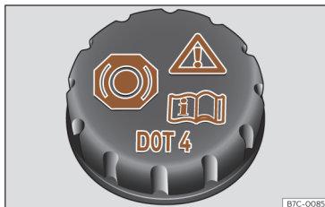
Fig. 227 Front compartment: brake fluid reservoir cap.
