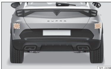
Fig. 134 Rear view of the vehicle: radar sensor areas.
