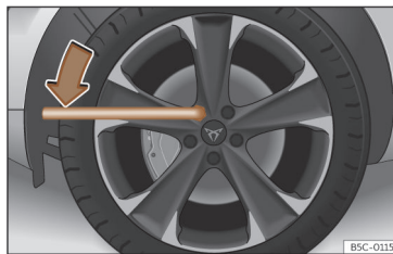
Fig. 195 Tyre change: loosen the wheel nuts.
