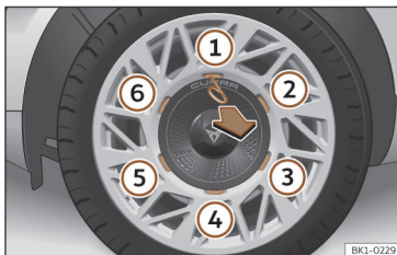
Fig. 192 Changing the wheel: removing the central trim.
