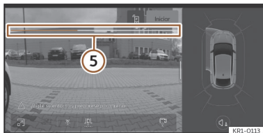
Fig. 139 On the infotainment system display: progress bar
