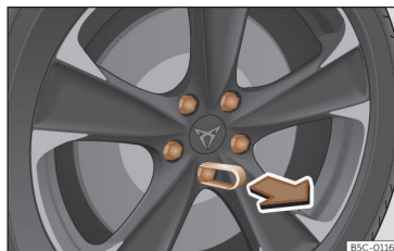
Fig. 193 Wheel: wheel nuts with caps.
