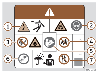
Fig. 51 High-voltage battery warning lettering.
