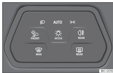
Fig. 93 Instrument panel: light panel.
