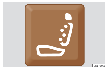
Fig. 92 On the lateral underside of the driver and passenger seats: massage function button.
