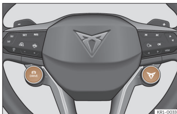
Fig. 108 Multifunction steering wheel: DRIVE and CUPRA buttons for selecting and changing the driving profile.
