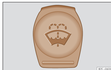
Fig. 188 In the front compartment: blue cap of the windscreen washer tank.
