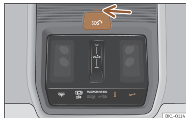
Fig. 46 On the roof console: controls for voice services.
