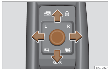
Fig. 99 Driver's door detail: exterior mirror control.
